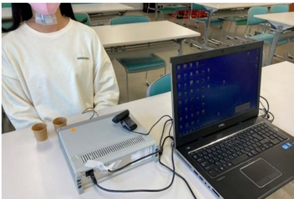
Figure 1. Swallowing test device. The device consists of 3 parts (i.e., a personal computer and 2 film sensors) and an interposer.
