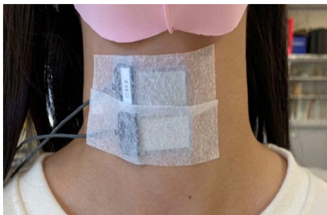
Figure 3. The attached film sensors. For collecting the swallowing data, 1 film sensor is attached to the hyoid bone (upper part), and the other is attached to the thyroid cartilage (lower part).
